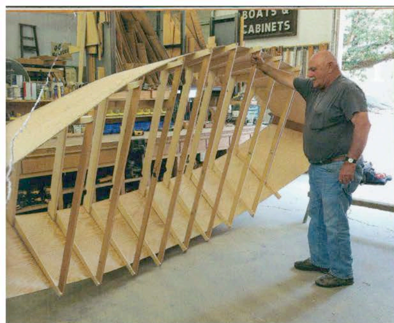
Steve Steele lifting a 16' x 48" drift boat that he is building. The lightweight wood drift boat dates back to the 1920s when Veltie Pruitt had his wood milled to his thinner specified dimensions to save weight.
